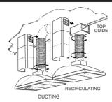
WARNING: The distance between the hob and the mounting holes of the canopy to be at least 900mm to ensure that the fully installed canopy has a clearance of 700mm (recommended height) between the lower part of the hood and the cooking hob. Before drilling any holes check the wall and the ceiling are clear of any electrical cables, pipes etc. Fixing to a solid stud is recommended. (A)
